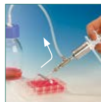
Aspiration with reverse modus valve
