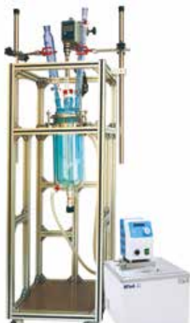
Ex. Multi-use High Temp. Bath Circulator with Modular Reactor System
