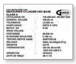
Each cylinder includes a batch calibration certificate. Cylinders on this page are calibrated to contain.
