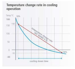
According to Newton's law of cooling, the rate of temperature change follows an exponential curve. The rate of temperature change calculated according to IEC 60068-3-5 applies to cooling from 90 % to 10 %. In the upper temperature range, the rate of temperature change is significantly higher, in the lower temperature range it is significantly lower.
