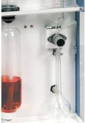
Automatic termination of final distillation at 200 ml of distillate. By using the ADD function small quantities of distillate can be added to accurately fill the matrix flask to the mark without having to add water to the distillation.
