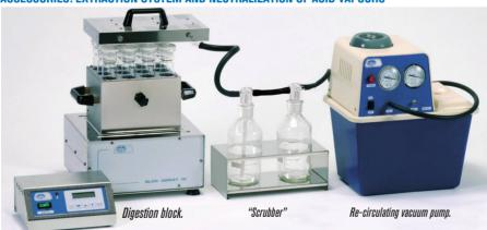
Specially designed to absorb and neutralize vapours generated in the Kjedahl digestion processes
