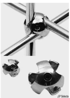
OIRIGINAL BOSSHEAD "TREVINGE" Made of chrome plated "Dural" alloy. Due to its strength, it is suitable for multilevel and three dimension constructions. Part No. 7008133 For Ø of 9 to 13 mm. Part No. 7008253 For Ø of 19 to 25 mm.
